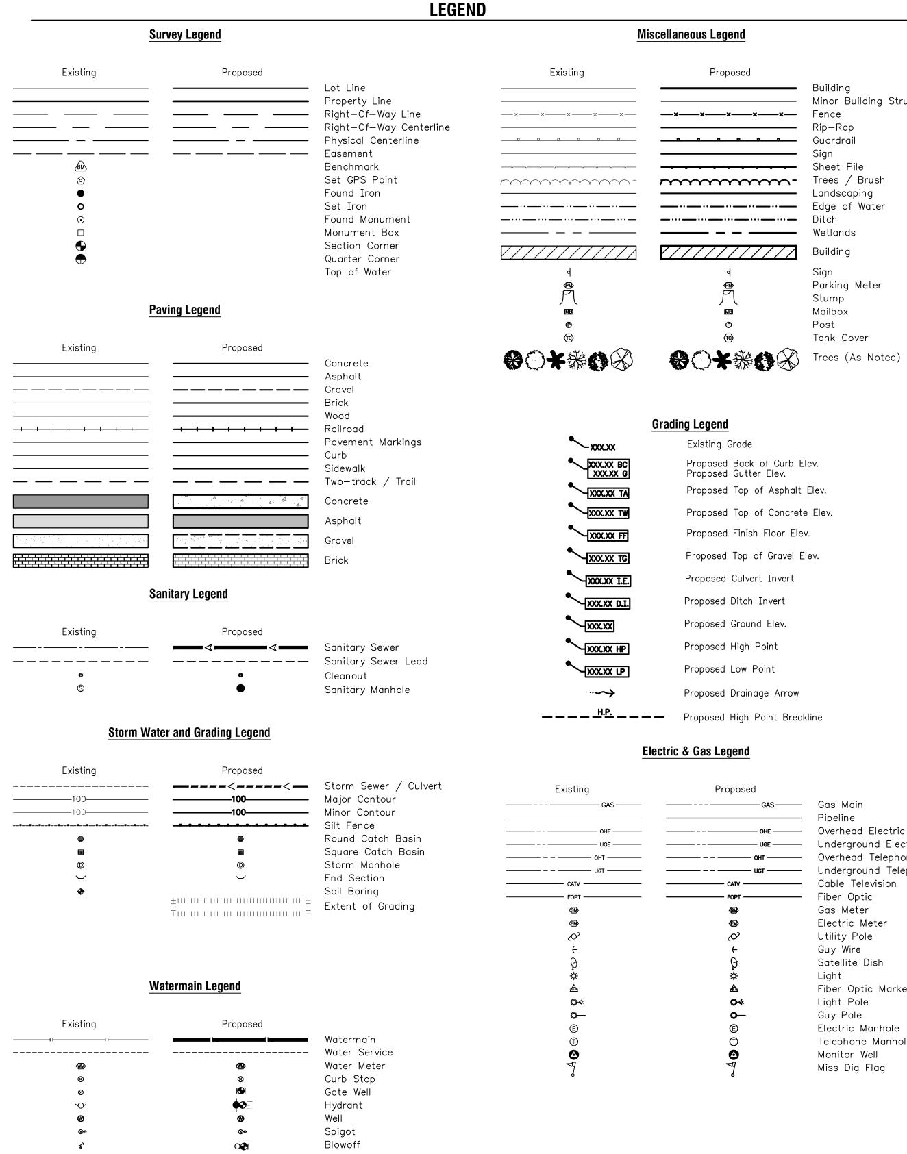
Proposed \_\_\_\_\_x\_\_\_\_x\_\_\_\_x\_\_\_\_\_x\_\_\_\_ ----- Sheet Pile ------ Edge of Water \_\_\_\_\_. Post 80×\*08
